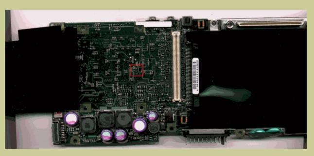
Then simply solder together the two pads as showing in the picture below and your L100 will go to 266MHz.
